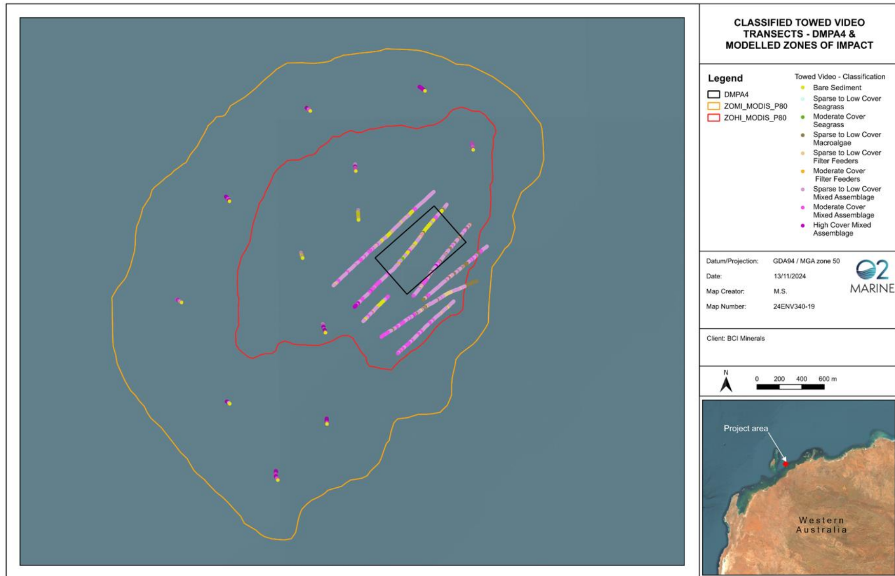
Figure 12: Towed video data across DMPA4 and within the predicted zones of impact (ZoMI, ZoHI)
