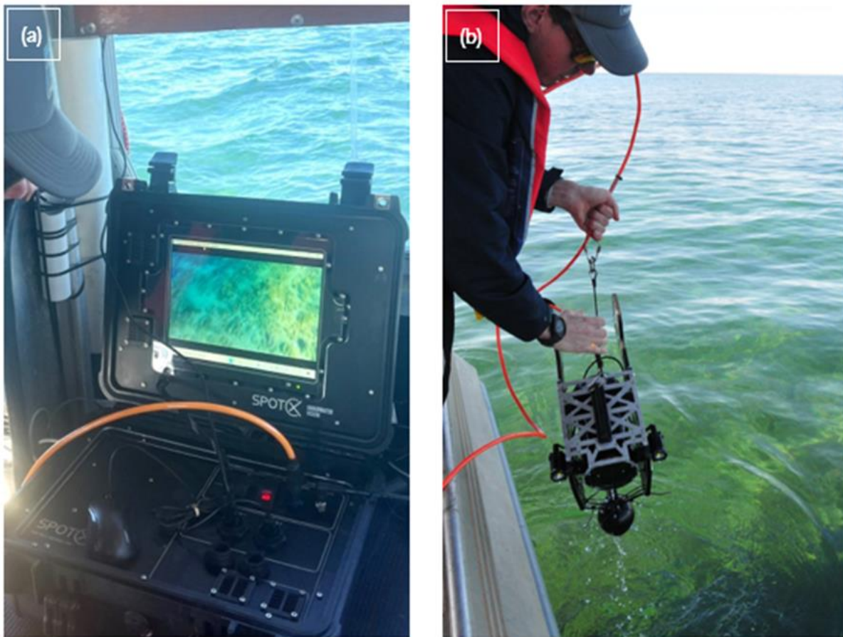
Figure 7: a) Spot X topside unit, and b) Spot X HD video camera and umbilical cable
