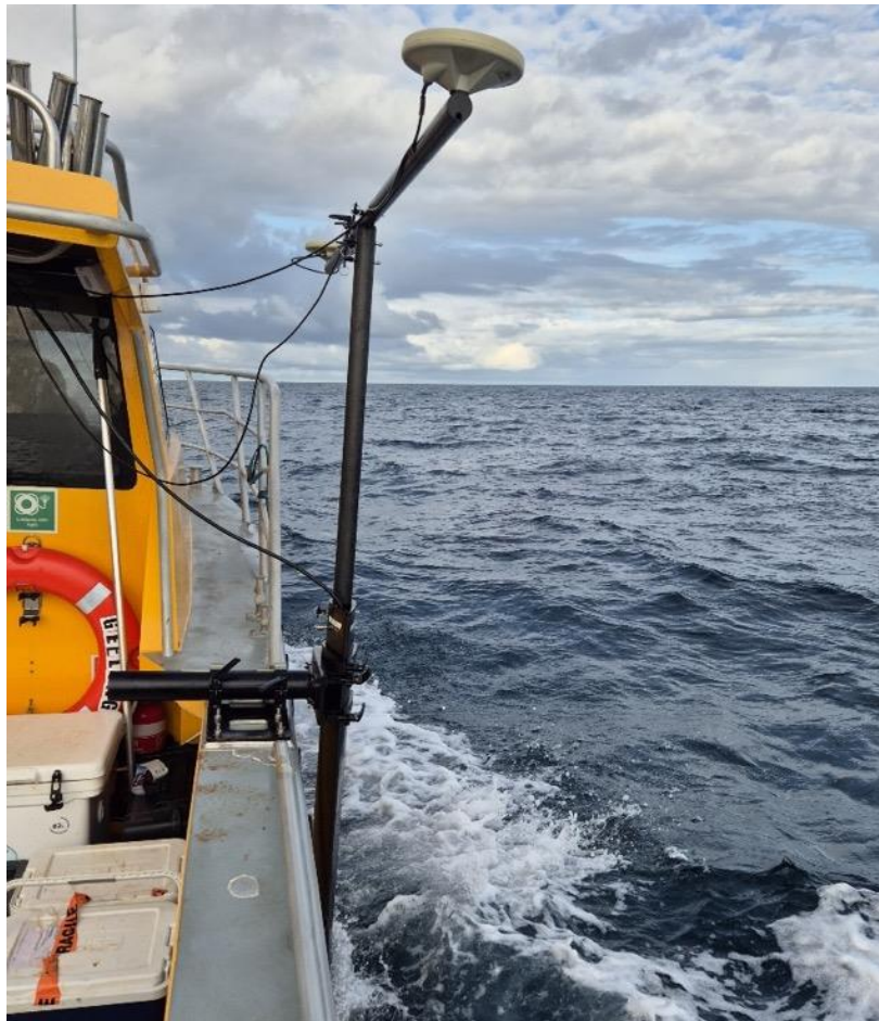
Figure 5: MBES side-mounted survey pole with integrated GNSS antenna supports.
