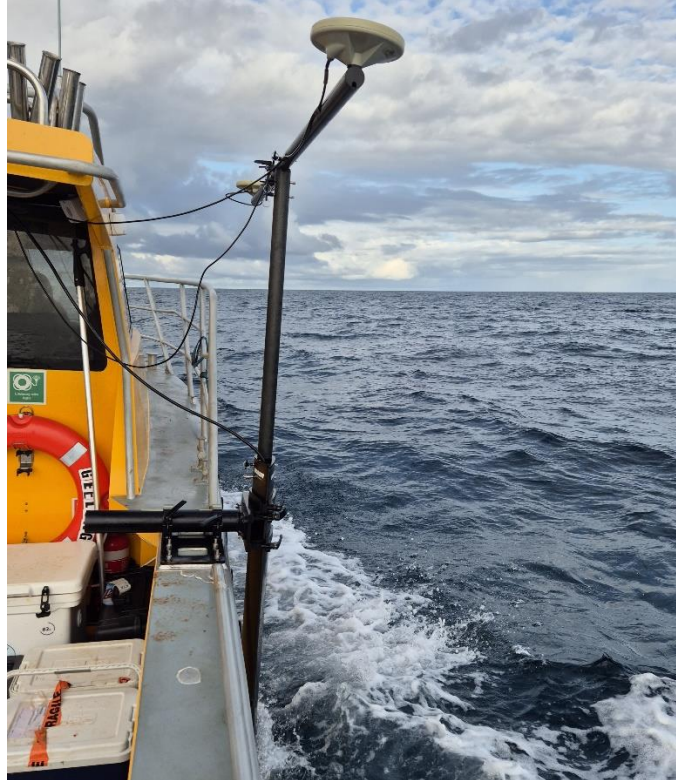
Figure 2 MBES side-mounted survey pole with integrated GNSS antenna supports.
