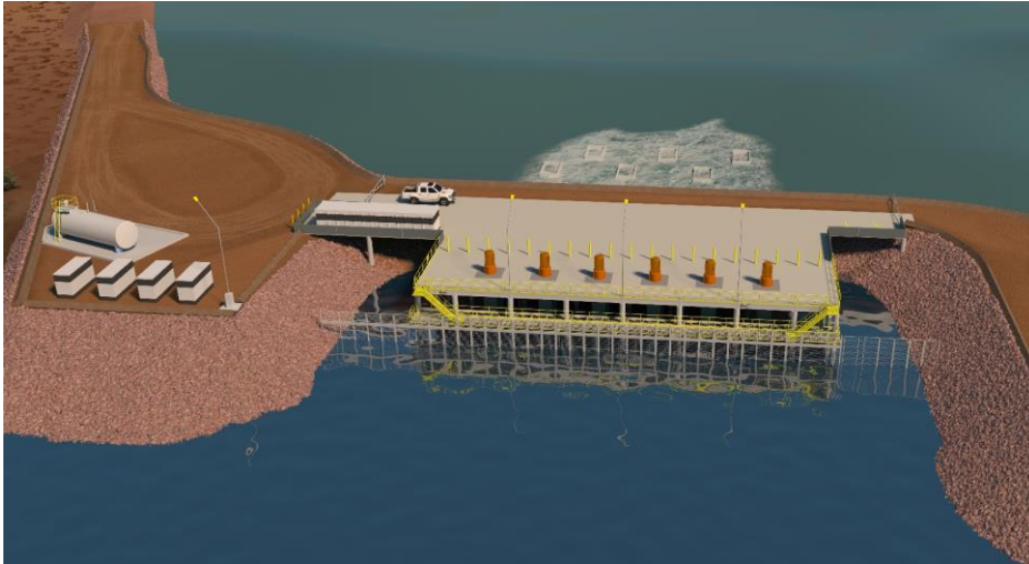
1. MAIN SEAWATER PUMP STATION
