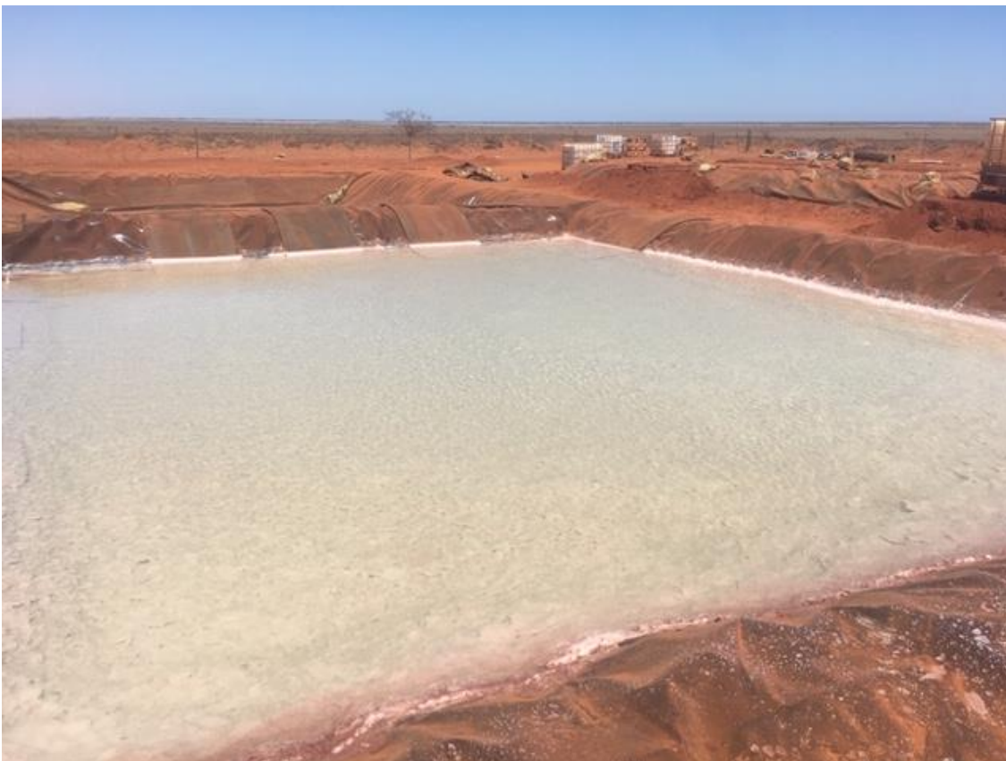
Figure 1: Raw salt crystallising in the small-scale Evaporation Ponds
