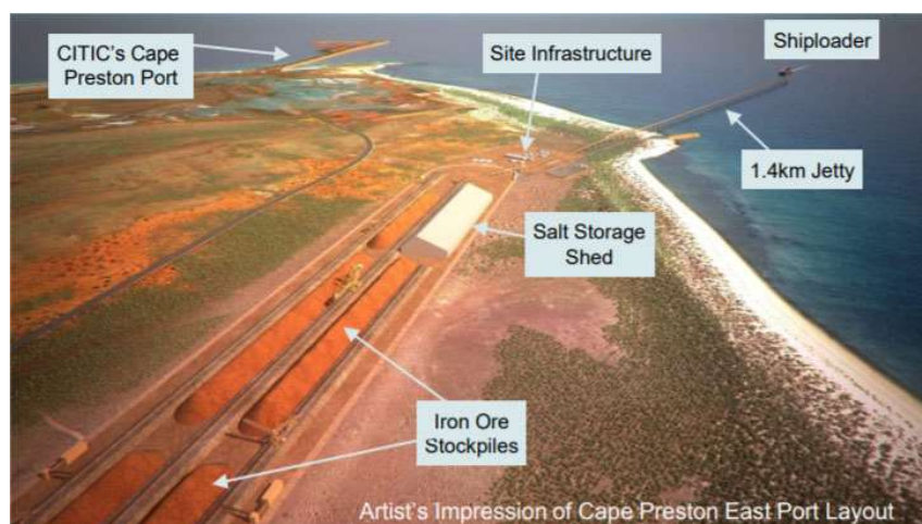
Figure 8. Cape Preston East proposed multi-commodity port facility (Source: Company).
