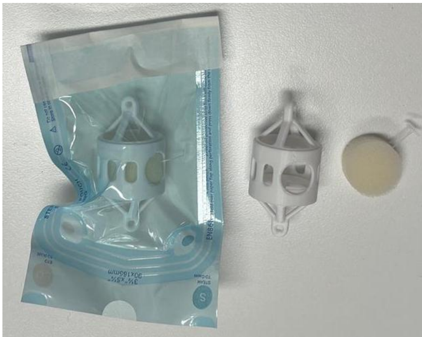
Figure 7: Example of the eDNA passive arrays - sample kit bag (LHS) and the pieces individually (RHS)
